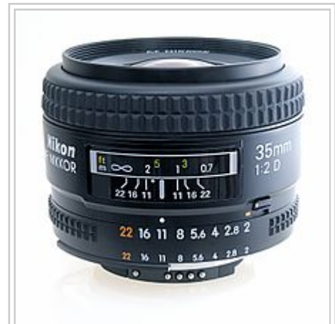
A 35 mm lens set to f/11 . The depth-of-field scale (top) indicates that a subject which is anywhere between 1 and 2 meters in front of the camera will be rendered acceptably sharp. If the aperture were set to f/22 instead, everything from just over 0.7 meters almost to infinity would appear to be in focus.
